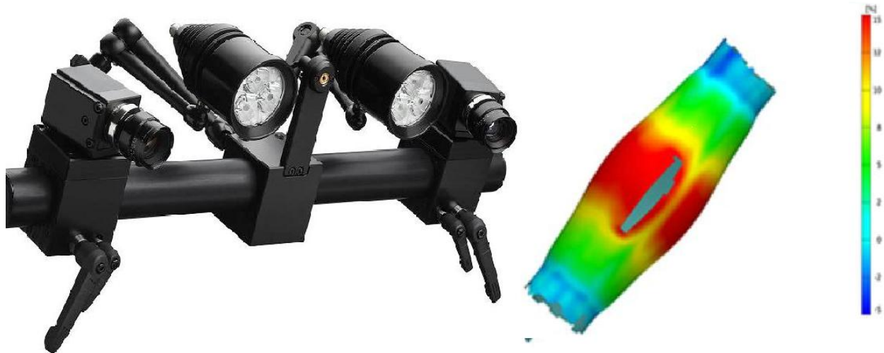
Fig. 2: Vibration Modes on a Tubular Structure
