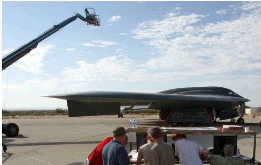
Fig. 9: ARAMIS Thermography from a boom overlooking the B2 Aft Deck c/o AFRL
