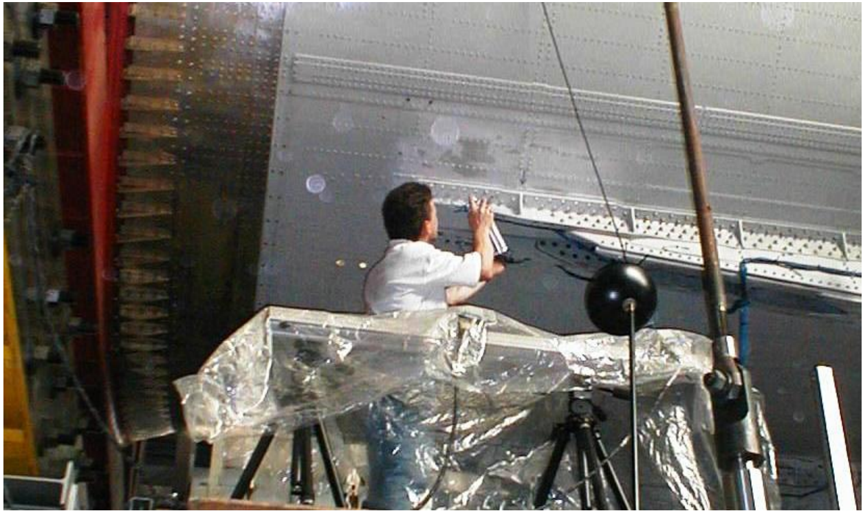
Fig. 1: Preparation for Strain Test of Riveted Area of Aircraft
