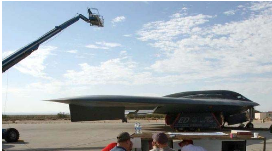
Figure 6 - ARAMIS Thermography from a boom overlooking the B2 Aft Deck c/o AFRL
