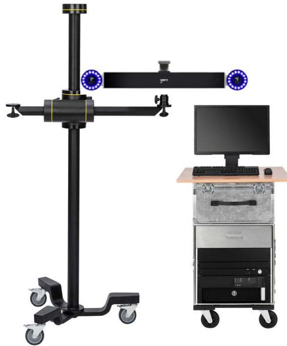
Figure 1 – Typical 3D-DIC system showing integrated stereo cameras with pulsed lighting for vibration studies, and a rack-mounted computer with data logger.
