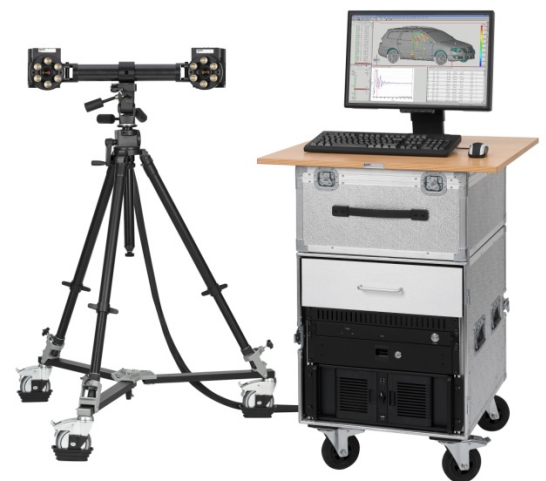
Figure 4 - ARAMIS system with sensor on tripod and mobile measurement station for structural measurements.
