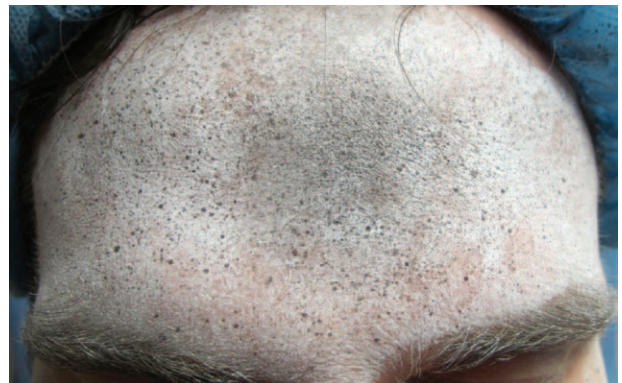
Fig. 1. A subject prepared for imaging. White foundation and black speckle makeup are applied to each patient. The speckles are tracked by the digital camera, and their displacement is quantified with ARAMIS.
