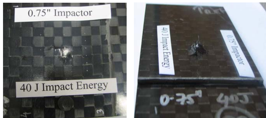
Figure 49. Impact Damage Induced on CFPW With 0.75-Inch Impactor
