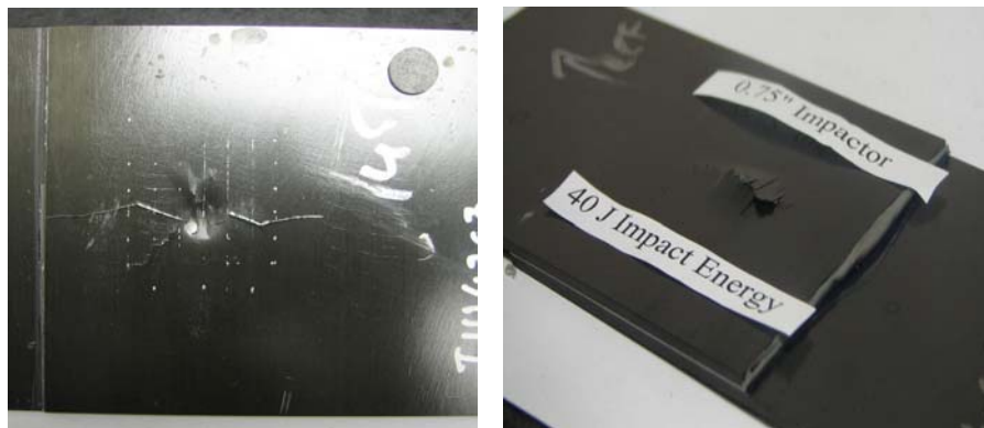
Figure 52. Impact Damage Induced on CFUT With 0.75-Inch Impactor
