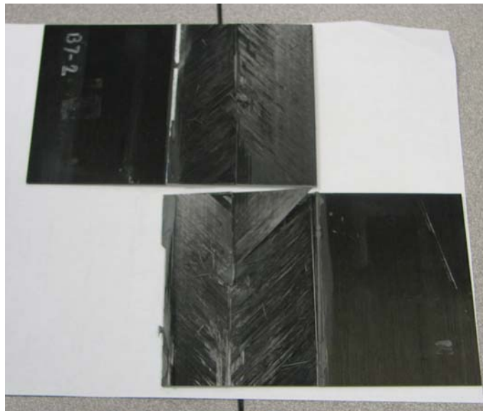
Figure 65. Typical Failure Mode Observed for CFUT SLS Specimens
