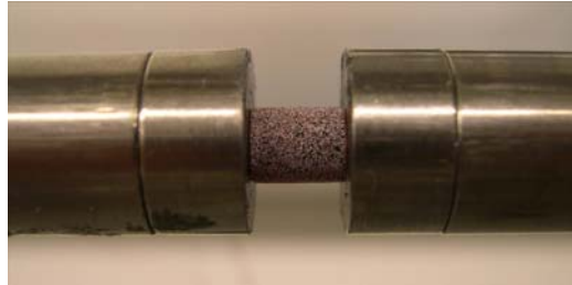
Figure 3: A patterned copper specimen in the compression SHB apparatus.
