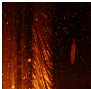
Figure 20: Post-test photo showing "orange peel" surface deformations in the notched region (non-painted area).
