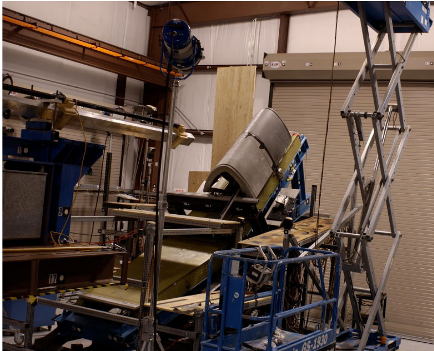
Figure 2: Wide angle view of ballistic impact setup for Orbiter leading edge panel 9 test series. RCC panels are mounted to wing leading edge on a massive test stand. The rectangular aluminum gun barrel extends towards the left edge of the photo.
