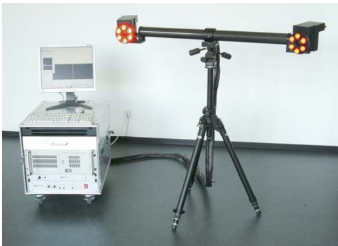
Figure 7 - Photogrammetry system measuring the response of multiple automobile engine components during startup.
